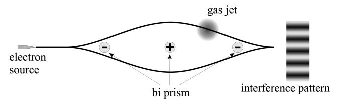
FIG. 1. Schematics, not to scale, of a biprism electron interferometer [14,15] adapted to measure the forward-scattering amplitude. Charged wires act as biprisms. The negatively charged wires split/recombine the beam and the positively charged wire redirects the two beams back together. The refractive index of a gas is measured by inserting a gas cell or a gas jet in one arm of the interferometer.
