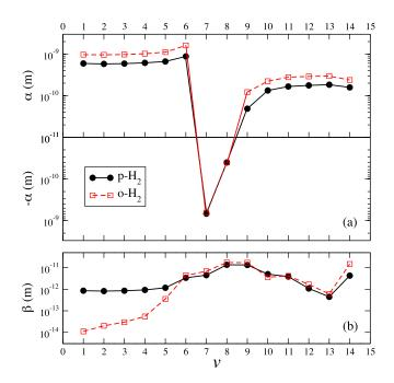
FIG. 1 (color online). Real component  $\alpha$  (top panel) and imaginary component  $\beta$  (bottom panel) of the complex scattering length for H<sub>2</sub> + H<sub>2</sub> collisions for initial state (v, j; v, j). Filled circle: para-H<sub>2</sub>, j = 0; open square: ortho-H<sub>2</sub>, j = 1. The value of  $\beta$  is dominated by QRVV transitions to (v + 1, j; v - 1, j) for all v.
