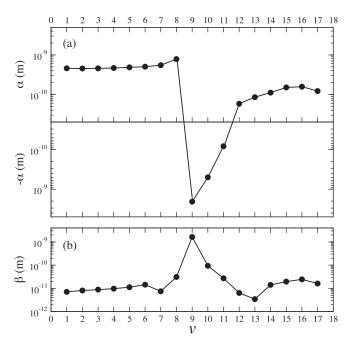
FIG. 6. Same as Fig. 2 except for HD + HD collisions for initial state (v, 0; v - 1, 2). The value of  $\beta$  is dominated by QRRR transitions to (v, 2; v - 1, 0) for large v, and the zero-energy resonance is located between that of the H<sub>2</sub> + H<sub>2</sub> and D<sub>2</sub> + D<sub>2</sub> cases.
